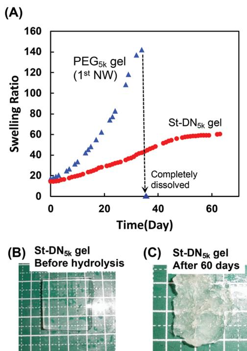
**Fig. 6** (A) Time course of swelling ratio during degradation test for 4-arm-PEG/PEG-DA (1<sup>st</sup> NW) gel and St-DN gel in PBS (pH = 7.4) at 37 °C. (B) and (C): photographs for St-DN gel before hydrolysis test and after 60 days, respectively.
