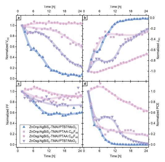
Fig. 2 Photovoltaic evolution in dry air with continuous 1 sun illumination of  $AgBiS_2$  NC solar cells with different extraction layers. The photovoltaic parameters, (a)  $V_{OC}$ , (b)  $J_{SC}$ , (c) FF and (d) PCE, were averaged from several devices and normalized to their initial value. A guide for the eye in form of a line is added.
