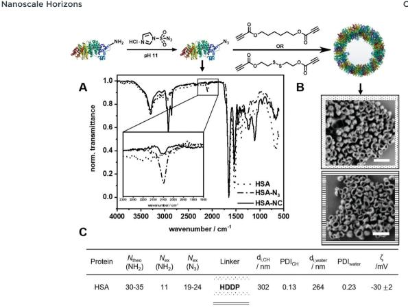
Fig. 2 Reaction scheme for the formation of protein nanocarriers through azide-alkyne click reaction (top). (A) IR spectra of native (...), azidefunctionalized (---) and human serum albumin nanocarriers (—). (B) SEM images of HSA-NCs using a HDDP (□) and HDDP-SS (□) ratio (Scale bar: 0.5 μm). (C) Analytic data of HSA NCs using HDDP and HDDP-SS.
