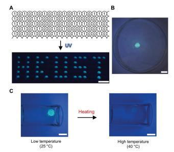
Fig. 10 Application of molecular logic operations. (A) Storage of a 'HKUST' pattern with 'Buffer (2)' gate matrices in a 384-well plate. Top: Schematic illustration of '0' or '1' input to wells. Bottom: Fluorescent pattern 'output'. (B) Solidification of logic gates in a dextran hydrogel. (C) Application of (B) as thermo-sensors in solution. A 365-nm UV lamp was used for excitation. Scale bars, 10 mm.
