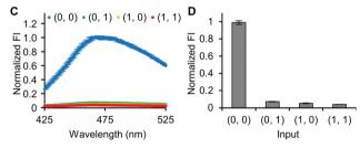
Fig. 7 NOR logic operation. (A) Symbol of logic gate. (B) Truth table. (C) The normalized fluorescence spectra of logic operation with different inputs. (D) Normalized FI at 471 nm. The concentrations of DCH and BSBOTPE used are 6  $\mu$ M and 141  $\mu$ M, respectively. Excitation wavelength was set at 350 nm. The 'heat' input is incubation under 40 °C for 2 min. The 'NaCl' input is increasing NaCl concentration from 150 mM to 600 mM, followed by 2-min incubation. n=3.
