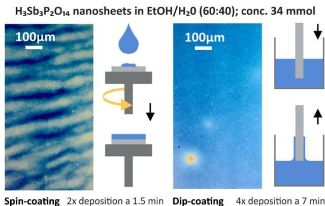
Fig. 3 Comparison of  $\text{H}_3\text{Sb}_3\text{P}_2\text{O}_{14}$  nanosheet-based thin films obtained by spin- (left) and dip-coating (right) including microscope images, the used parameters and schematic descriptions of both processes.
