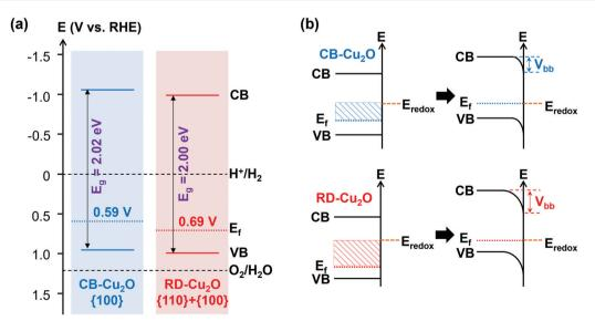
Fig. 4 (a) Postulated electronic band structures and (b) expected downward band bending at the semiconductor/electrolyte junctions of CB-Cu<sub>2</sub>O and RD-Cu<sub>2</sub>O
