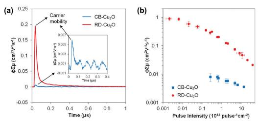
Fig. 6 (a) TRMC signal of CB-Cu<sub>2</sub>O and RD-Cu<sub>2</sub>O over time at  $7.0 \times 10^{12}$  photons pulse<sup>-1</sup> cm<sup>-2</sup>, with the inset showing the magnification of the signal of CB-Cu<sub>2</sub>O, and (b) maximum TRMC signal as a function of incident pulse intensity of CB-Cu<sub>2</sub>O and RD-Cu<sub>2</sub>O.
