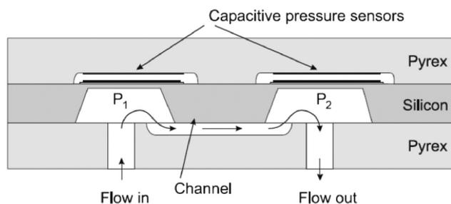
Fig. 4 Differential pressure flow rate sensor with capacitive readouts.<sup>55</sup>
