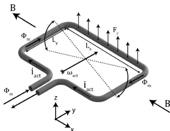
**Fig. 3** Representation of the Coriolis flowmeter principle: the channel rotates periodically around the  $y$  axis with an angular velocity  $\omega_{\text{act}}$ . When a mass flow  $\Phi_m$  flows through the channel, a Coriolis force  $F_c$  will cause a secondary vertical motion.<sup>118</sup>
