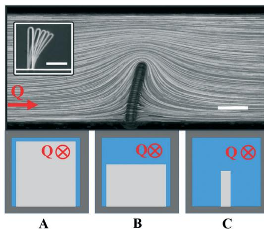
Fig. 5 On the top: Bending of a cantilever under flow with seeded particles, adapted from Wexler *et al.*<sup>69</sup> At the bottom: The different confinement degrees of the cantilever-based flowmeters: A-the cantilever is fully confined, B-the cantilever is only confined along one direction, C-the cantilever is not confined.
