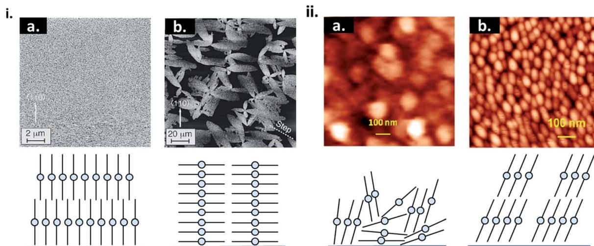
**Fig. 6** (i) AFM images CuPc thin-films and cross sectional diagrams CuPc molecules deposited on (a) rough and (b) smooth Si(111)–H surfaces. Adapted with permission from ref. 43. Copyright© 1996 American Vacuum Society. (ii) AFM images of CuPc thin-films and diagrams of CuPc molecules deposited on (a) bare  $\text{SiO}_2$ , and (b) OTS treated  $\text{SiO}_2$ . Adapted with permission from ref. 49. Copyright© 2015 American Chemical Society.
