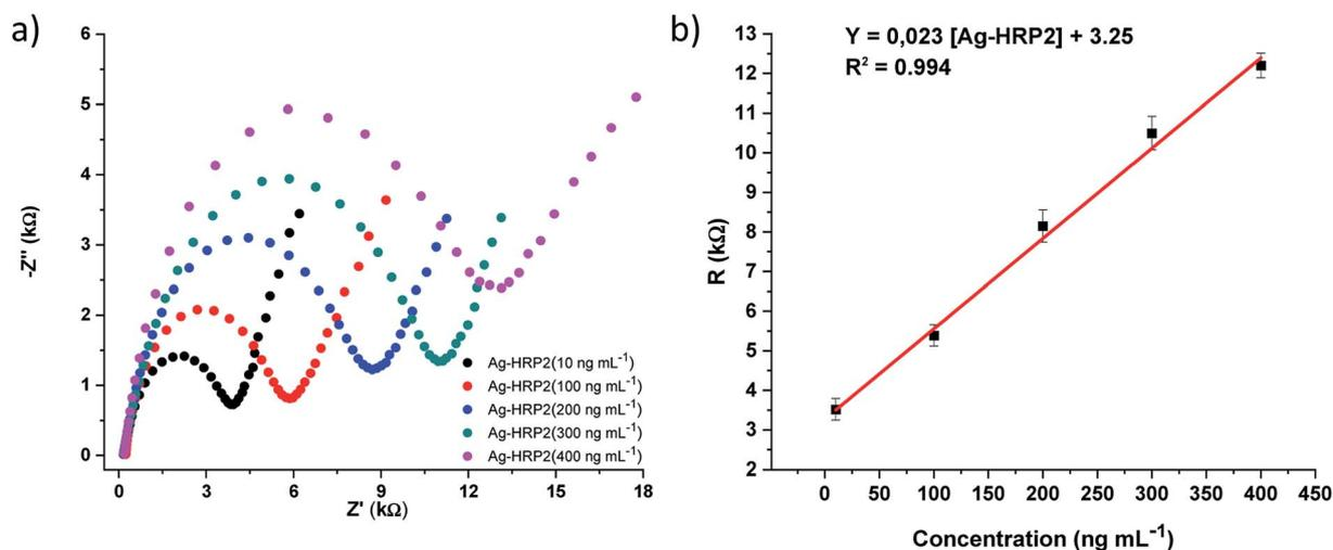
Fig. 5 (a) EIS spectra recorded with the Ab-PfHRP2/DHP/GE electrochemical immunosensor upon additions of Ag-PfHRP2 (10, 100, 200, 300, and 400 ng mL<sup>-1</sup>), (b) calibration curve:  $Y = 0.023 [\text{Ag-PfHRP2}] + 3.25$ , with an  $R^2 = 0.994$ .
