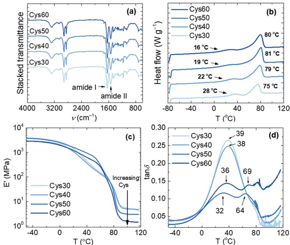
Fig. 2 Characterization of the PA CANs; (a) FTIR spectra, (b) DSC traces of the 2<sup>nd</sup> heating scan and (c), (d)  $E'$  and  $\tan \delta$ , respectively, from DMA analysis.
