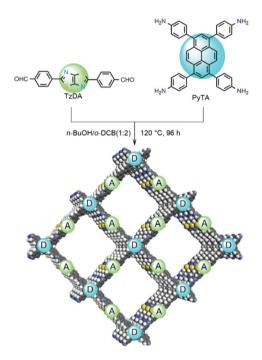
Fig. 8 Donor–Acceptor (D–A) MOF system synthesized under solvothermal condition. This figure has been reproduced from ref. 145 with permission from John Wiley and Sons, copyright 2021.
