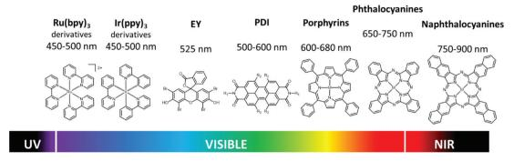
Fig. 2 Examples of PS molecules covering the Vis-NIR absorption window. The optical properties can be finely tuned by changing the substituents or the central metal (in the case of porphyrins, phthalocyanines and naphthalocyanines. The choice of the substituents affects also the solubility, aggregation properties, and the interaction with the different photocatalytic materials.
