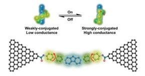
Fig. 9 Schematic of conformational transition of terphenyl units between strongly conjugated and weakly-conjugated states and corresponding hexaphenyl aromatic chain single-molecule junctions. Reprinted with permission from Xin et al., Nano Lett., 2017, 17, 856. Copyright 2017 American Chemical Society.
