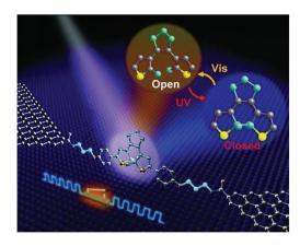
**Fig. 8** Schematic of a graphene-diarylethene-graphene junction that highlights the expansion of the molecular bridge by methylene groups. Reprinted with permission from Jia et al., Science, 2016, **352**, 1443. Copy right 2016 AAAS.
