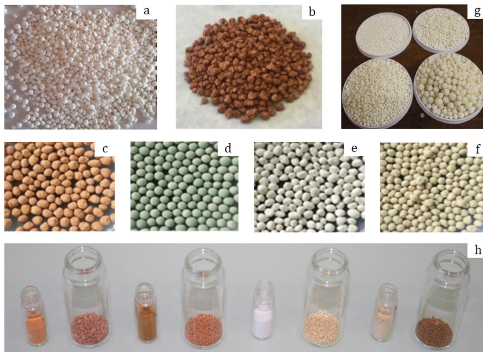
Fig. 5 Photographs of: MIL-160 granules (a) prepared by Permyakova et al. 67 Copyright 2017 Wiley. MIL-100 granules (b) prepared by Martins et al. 69 Copyright 2020 American Chemical Society. MIL-100 (c), MIL-101 (d), UiO-66 (e), and UiO-66-NH 2 (f) containing 5 wt% MRA binder prepared by Valekar et al. 57 Copyright 2017 The Royal Society of Chemistry. UiO-66 granules (g) prepared by Ren et al. 73 Copyright 2015 Elsevier. MIL-100, MIL-127, UiO-66, and UiO-66-NH 2 granules (h, from left to right in big vessels) with their corresponding powders in small vessels prepared by Chanut et al. 71 Copyright 2016 Wiley.
