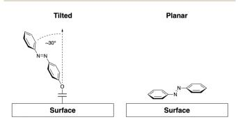
Fig. 1 A representation of common surface interactions. Angled SAM arrangement with an example angle to the normal of  $\sim 30^{\circ}$  (left-hand side)<sup>61</sup> and planar or "face on" adsorption common for unfunctionalized azobenzene (right-hand side).74,75
