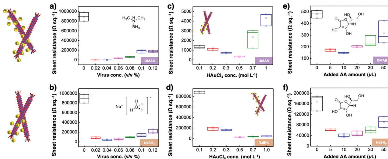
Fig. 2 Sheet resistance according to (a) and (b) virus concentrations, (c) and (d) HAuCl<sub>4</sub> concentrations, and (e) and (f) AA concentrations under DMAB and NaBH<sub>4</sub> reducing agents.
