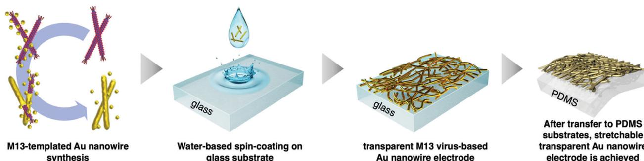
Fig. 1 Schematic illustration of the growth, thin-film fabrication, and transfer of the M13 bacteriophage-templated gold nanowire for stretchable electrode applications.
