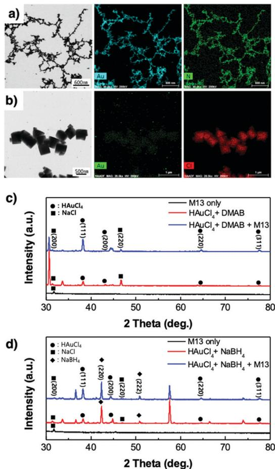
Fig. 3 STEM images and EDS analysis of the virus-templated Au nanowires formed under (a) DMAB and (b)  $\text{NaBH}_4$ . XRD spectra of the virus-templated Au nanowires formed under (c) DMAB and (d)  $\text{NaBH}_4$ .
