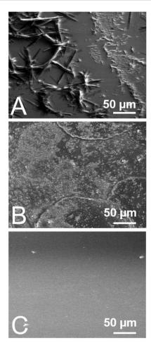
Fig. 3 SEM images of self-doped PDI (compound #2) (A) drop-cast (B) ultrasonically sprayed and (C) vapor deposited into thin films.
