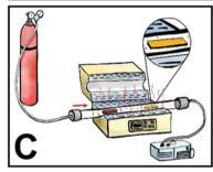
Fig. 2 Depiction of the three thin film processing methods investigated. (A) Drop-casting and dried in air at room temperature. (B) Ultrasonic spray coating onto heated substrates. (C) Physical vapor deposition in a tube furnace under vacuum
