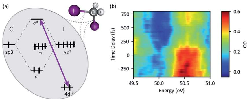
**Fig. 9** (a) Term scheme of the diiodomethane ( $\text{CH}_2\text{I}_2$ ) target molecule. The resonant XUV excitation from the iodine 4d orbital to an antibonding  $\sigma^*$  molecular orbital is indicated by the violet arrow. (b) XUV-pump XUV-probe transient absorption spectroscopy of diiodomethane (probe-pulse spectrum).
