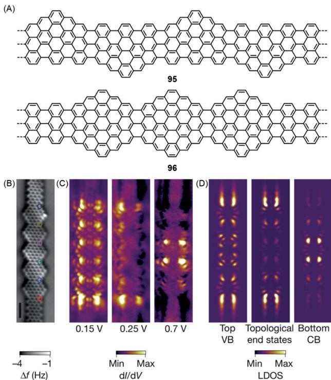
Fig. 17 (A) Chemical structures of GNRs **95** and **96** with topological phases. (B) Constant-height nc-AFM image of GNR **96** on Au(111). (C) Experimental and (D) simulated  $dI/dV$  maps of GNR **96** on Au(111).<sup>43</sup> Copyright 2018. Adapted with permission from Macmillan Publishers Ltd: Nature.
