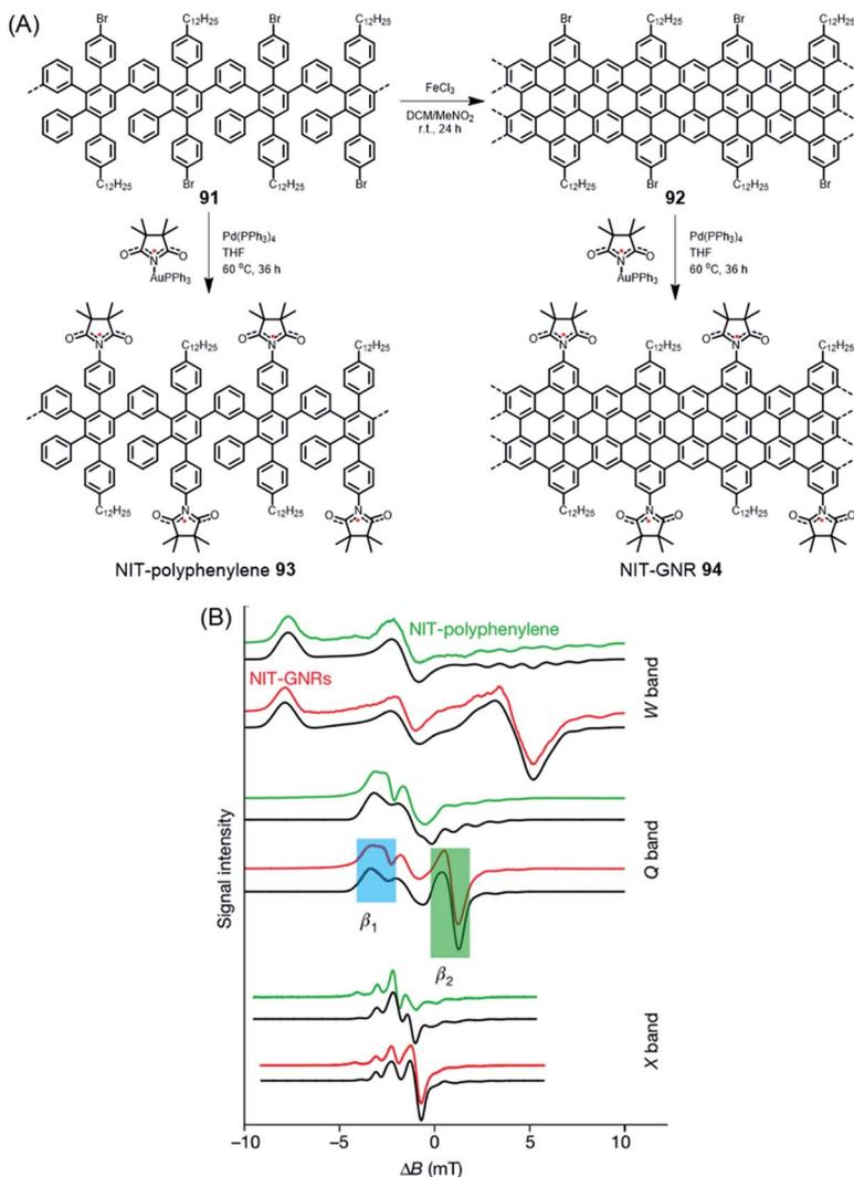
Fig. 16 (A) Synthetic route for NIT-polyphenylene **93** and NIT-GNR **94**. (B) Multifrequency ESR spectra for NIT-polyphenylene **93** (green) and NIT-GNR **94** (red), along with simulations (black), plotted against the magnetic field from the edge-state resonance.<sup>146</sup> Copyright 2018. Adapted with permission from Macmillan Publishers Ltd: Nature.
