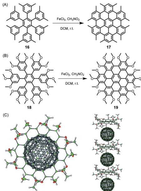
Fig. 3 Synthetic route to (A) dodecamethyl HBC **17** and (B) octadecamethoxy HBC **19**; DCM = dichloromethane. (C) Single-crystal structure of the complex formed between fullerene and **19**: top view and side view of the columnar packing arrangement.<sup>82</sup> Copyright 2005. Adapted with permission from WILEY-VCH Verlag GmbH & Co. KGaA, Weinheim.
