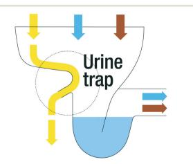
Fig. 2 Basic principle of urine-separating flush toilets using the teapot effect. Copyright EOOS.
