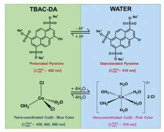
Fig. 3 Structures of various forms of pyranine and Co<sup>II</sup> based on the solubilizing media
