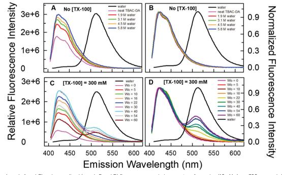
Fig. 4 Relative (panels A and C) and normalized (panels B and D) fluorescence emission spectra of pyranine (10  $\mu$ M,  $\lambda_{ex}$  = 390 nm, and slits: excitation/ emission = 2/2 nm) dissolved within neat DES TBAC-DA and TX-100(300 mM)/TBAC-DA systems at different amounts of water loading (w<sub>0</sub>), respectively. The fluorescence emission spectrum of pyranine in water is also included in each panel for reference.
