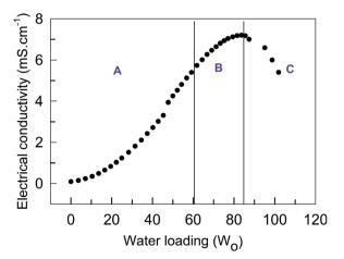
Fig. 7 Electrical conductivity (mS cm<sup>-1</sup>) as a function of water loading  $(w_0)$  in water/TX-100 (300 mM)/TBAC-DA microemulsion at ambient conditions. Regions A, B, and C are described in the text.
