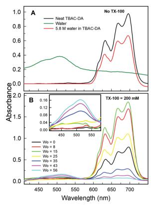
Fig. 5 UV-vis absorption spectra of Co<sup>II</sup> within water, neat TBAC-DA, and water saturated TBAC-DA (panel A) and the TX-100 (200 mM)/TBAC-DA system (panel B) at different amounts of water loading  $(w_0)$ . Inset in panel B is the magnified portion of the plot for clear depiction of the peak at  $\sim$  509 nm.
