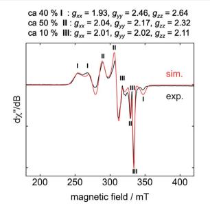
Fig. 2 EPR spectrum (–203 °C) of the reaction mixture of 1 with  $C_6F_6$  after 5 s at -78 °C in thf.
