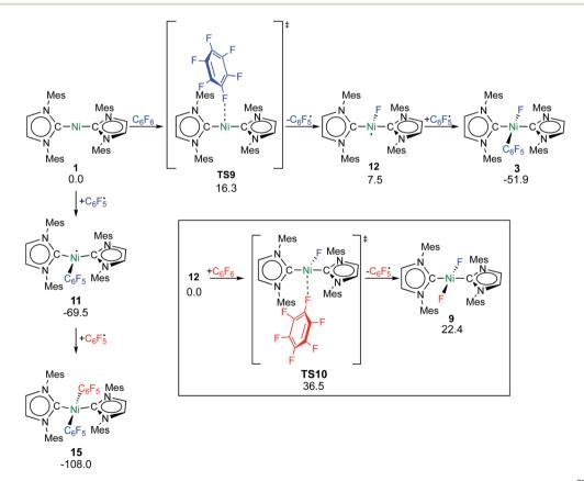
Scheme 10 Calculated pathways for the homolytic C-F bond cleavage of  $C_6F_6$  by 1 and further radical reaction steps ( $\Delta G^{298}$  in kcal mol<sup>-1</sup>; energies of TS10 and 9 are given relative to  $12 + C_6F_6$ ).
