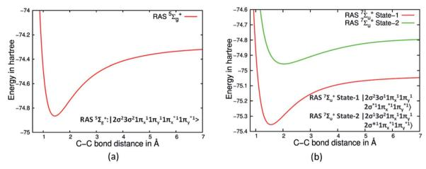
Fig. 3 (a) PEC corresponding to the RASSCF computation for the quintet spin state of  $C_2$  and (b) PECs corresponding to the RASSCF computation for the two septet spin states of  $C_2$  along with their dominant configurations.
