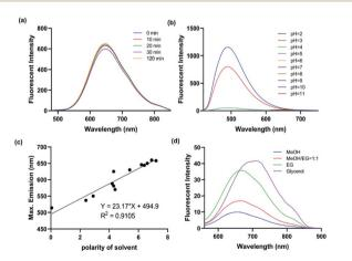
Fig. 2 (a) The fluorescent spectra changes of ICTAD-1 (10  $\mu$ M) in DMF under the irradiation of daylight lamp for 120 min; (b) the fluorescent spectra of ICTAD-1 (10  $\mu$ M) in different pH aqueous solutions (1% DMF); (c) the linear relationship between the polarity of solvent and the maximum emission wavelength; (d) the fluorescence spectra of ICTAD-1 (10  $\mu$ M) in solvents of different viscosity, EG: ethylene glycol.
