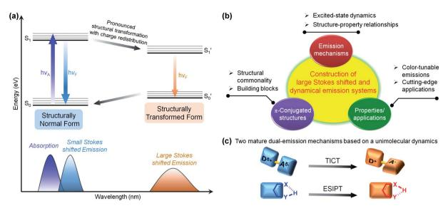
Fig. 1 (a) Jablonski diagram for the normal and transformed two-state model resulting in a large Stokes shift and dual fluorescence. (b) Route for the construction of a specific emission system and concept. (c) Illustrative schemes of two mature dual-emission mechanisms based on unimolecular dynamics: TICT and ESIPT.
