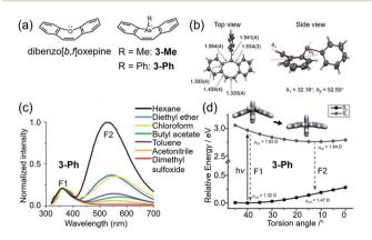
Fig. 5 (a) Chemical structures of dibenzo[b,f]oxepine and dibenzo[b,f] arsepin derivatives **3-Me** and **3-Ph**. (b) Single-crystal structure of **3-Ph**. (c) Photoluminescence spectra of **3-Ph** in various solvents. (d) Calculated potential energy surface of **3-Ph** with the variation in the torsion angle in the S<sub>0</sub> and S<sub>1</sub> states. Reproduced from ref. 101 with permission from the Wiley-VCH, Copyright 2019.
