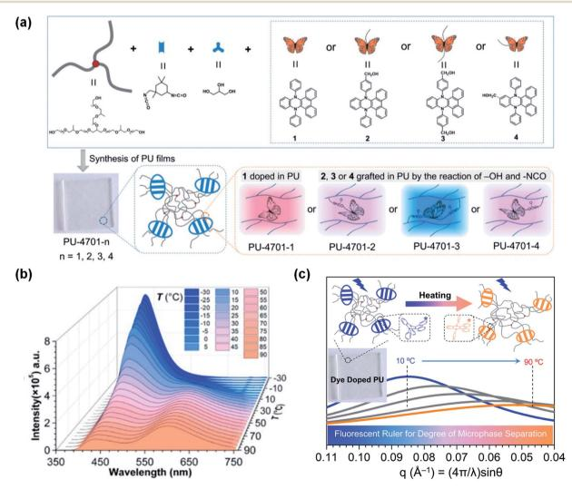
Fig. 9 (a) Diagrammatic sketch illustrating the DPAC-doped polyurethanes PU-4701-1-PU-4701-4. (b) PL spectra of PU-4701-2 at various temperatures (-30 to 90 °C). (c) Scattering curves of PU-4701-1 achieved by small-angle X-ray scattering at various temperatures (10-90 °C). Reproduced from ref. 107 with permission from the American Chemical Society, Copyright 2019.
