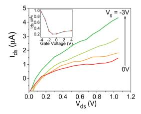
Fig. 2 Protonic FET measurement, source–drain current ( $I_{DS}$ ) as a function of the source–drain voltage ( $V_{DS}$ ) at different values of gate voltage  $V_{GS}$  for unmodified BSA mat. The inset shows the transfer line characteristics of the device.
