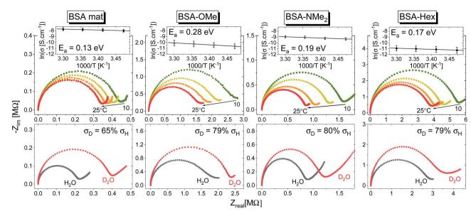
Fig. 7 (Top) Temperature dependence studies of the PC across the various BSA mats. The insets show the Arrhenius plot of the logarithmic of conductivity (averaged of at least 3 replicas) as a function of inverse temperature along with the calculated activation energy ( $E_a$ ). (Bottom) Kinetic isotope effect of the PC across the various BSA mats upon deuterating the sample along with the calculated decrease in measured conductivity upon deuteration.
