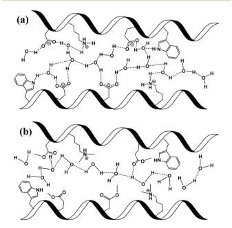
Scheme 2 Schematic representation of individual PT steps and general PC pathway in (a) unmodified BSA mat, where protons are mediated *via* the formation of hydrogen bonds between amino acid side chains and water molecules; and (b) in modified BSA, where the hydrogen bond network is disrupted and protons are less interacting with the side groups of the protein.
