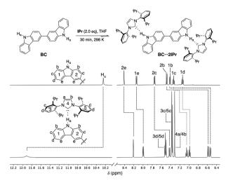
Fig. 2 Partial  $^1$ H NMR spectra (500 MHz, THF- $d_8$ ) of BC (50 mM) and BC...2IPr. Dashed lines indicate chemical shift changes upon hydrogen bonding to IPr.
