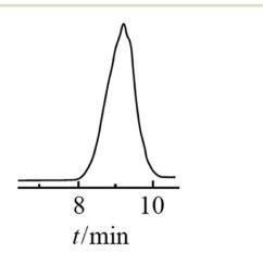
Fig. 20 GPC curve of the polyphenyl(ethoxy)siloxane obtained, MW = 1000.<sup>24</sup> Reproduced with the permission of Elsevier publishing.
