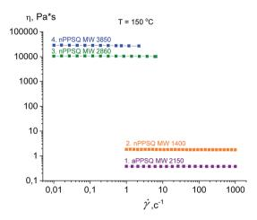
Fig. 33 Dependence of viscosity on the shear rate (flow curves) at 150 °C for the PPSQ obtained.<sup>25</sup> Reproduced with the permission of Elsevier publishing.
