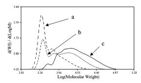
Fig. 16 Molecular weight distribution of the main hydrolysis products of phenyltriethoxysilane in the presence of the following catalysts: (a) – Me4NOH, (b) a mixture of Me<sub>4</sub>NOH with octylamine and (c) octylamine. Reprinted with permission from ref. 118. Copyright 2020 American Chemical Society.
