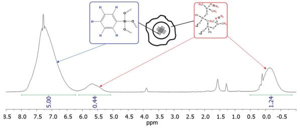
Fig. 29 <sup>1</sup>H NMR of the nanogel with a dimethylvinylsilyl shell obtained. <sup>141</sup>
