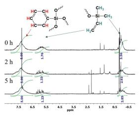
Fig. 26 <sup>1</sup>H NMR spectra of n-PPSQ blocked with dimethylvinylsilyl groups without preliminary condensation (1), as well as after condensation for 2 h (2) and 5 h (3).24 Reproduced with the permission of Elsevier publishing
