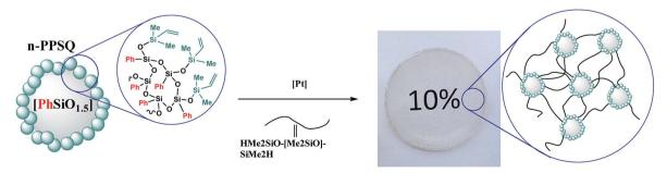
Fig. 27 Scheme of PDMS and n-PPSQ phenylated copolymer curing. 141 Reproduced with the permission of Elsevier publishing
