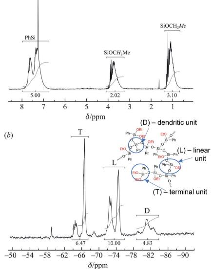
Fig. 21 (a)  $^{1}$ H and (b)  $^{29}$ Si NMR spectra of the polyphenylethoxysiloxanes obtained: D – trisubstituted silicon atom; L – disubstituted silicon atom; T – monosubstituted silicon atom.  $^{24}$  Reproduced with the permission of John Wiley and Sons.
