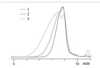
**Fig. 25** GPC curves of n-PPSQ blocked with dimethylvinylsilyl groups without preliminary condensation ((1) MW-1000), after 2 hours ((2) MW from 10 000 to 1200) and after 5 hours of condensation ((3) MW from 32 000 to 1500).<sup>24</sup> Reproduced with the permission of Elsevier publishing.
