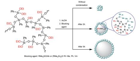
Fig. 24 Production of n-PPSQ with various core/shell ratios.<sup>24</sup> Reproduced with the permission of Elsevier publishing
