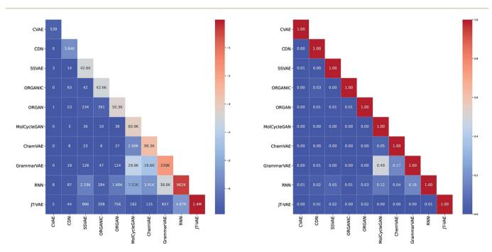
Fig. 3 (Left) The diagonal of the matrix illustrates total number of molecules generated by each method. Intersections below the diagonal show number of same molecules that were generated by both methods. (Right) Each entry shows the proportion of shared molecules between each method.
