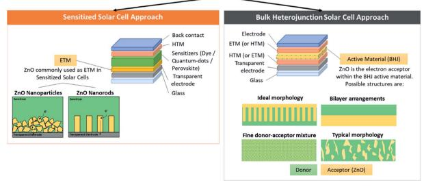
Fig. 2 Nanostructured ZnO in emerging solar cell applications.
