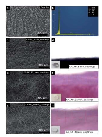
Fig. 3 (a) SEM image with (b) EDX analysis of bare Cu disk, SEM images of the Cu disk coatings CA-Nf after (c) 5 min (e) 15 min (g) 30 min coatings (d, f and h) photos of the coating thickness analysis.
