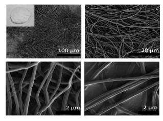
Fig. 2 SEM micrographs of pristine CA-Nf, Inset shows the photo of the pristine CA-Nf after electrospinning process.
