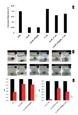
Fig. 7 Cu, Cu coated CA-Nf and Cu coated CA-Nf with 5% AgNps in the ASW and ASW inoculated with  $\it E.~coli$  (a) corrosion rates values (mm y $^{-1}$ ) (b) photographs of the Cu discs weight loss analysis and (c) pH changes.
