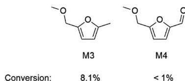
Scheme 5 The conversion of model compounds **M3** and 5-(methoxymethyl)furan-2-carbaldehyde (**M4**) in [BMIM]Cl with  $\text{CrCl}_3$  and water. Reaction conditions: [BMIM]Cl (0.5 g),  $\text{CrCl}_3$  (6.6 mg), substrate (0.5 mmol), water (20 mg),  $90^\circ\text{C}$ , 0.5 h, under air.
