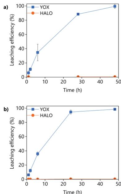
Fig. 5 Effect of the leaching time on the leaching efficiency of YOX and HALO using (a) LevA–ChCl and (b) levulinic acid. The leaching conditions are:  $T = 80\text{ }^{\circ}\text{C}$ ; L/S = 10; H<sub>2</sub>O vol% = 30; and 500 rpm.
