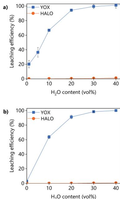
Fig. 4 Effect of the water content on the leaching efficiency of YOX and HALO using (a) LevA–ChCl and (b) levulinic acid. The leaching conditions are:  $T = 80\text{ }^{\circ}\text{C}$ ,  $t = 48\text{ h}$ , L/S = 10 and 500 rpm.
