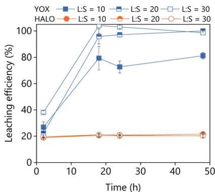
Fig. 10 Effect of the L/S ratio and leaching time on the leaching efficiency of a real lamp phosphor waste using the ionic liquid [Hbet][NTf<sub>2</sub>]. The leaching conditions are: H<sub>2</sub>O vol% = 5; T = 80 °C; 500 rpm.
