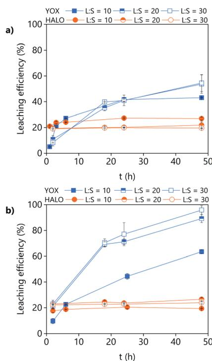
**Fig. 9** Effect of the L/S ratio and leaching time on the leaching efficiency of a real lamp phosphor waste using (a) LevA–ChCl and (b) levulinic acid. The leaching conditions are: H<sub>2</sub>O vol% = 30; T = 80 °C; 500 rpm.
