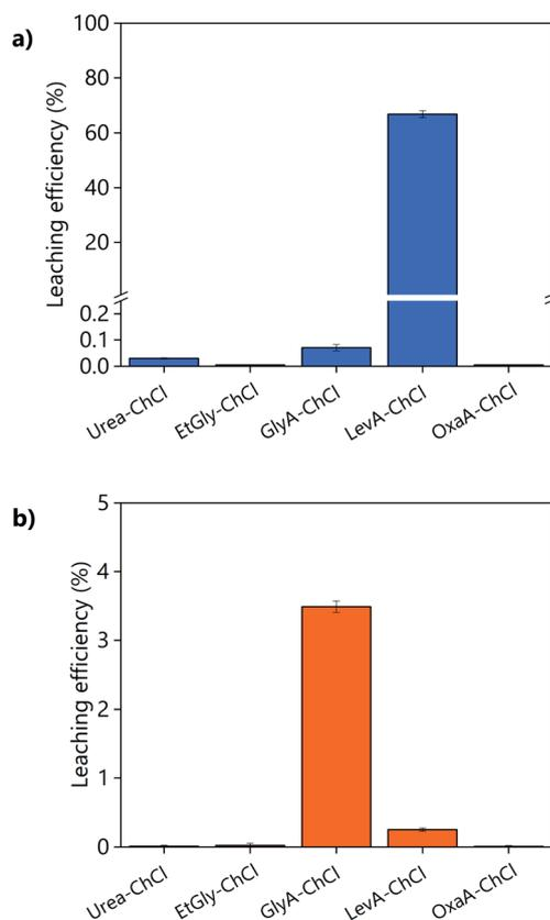
Fig. 2 Effect of the hydrogen-bond donor type on the leaching efficiency of (a) YOX lamp phosphor and (b) HALO lamp phosphor. The leaching conditions are: H<sub>2</sub>O vol% = 10; T = 80 °C; t = 48 h; L/S = 10 and 500 rpm.
