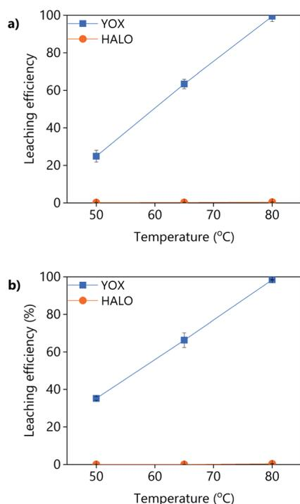
Fig. 6 Effect of the temperature on the leaching efficiency of YOX and HALO using (a) LevA–ChCl and (b) levulinic acid. The leaching conditions are: H<sub>2</sub>O vol% = 30; *t* = 48 h; L/S = 10; 500 rpm.
