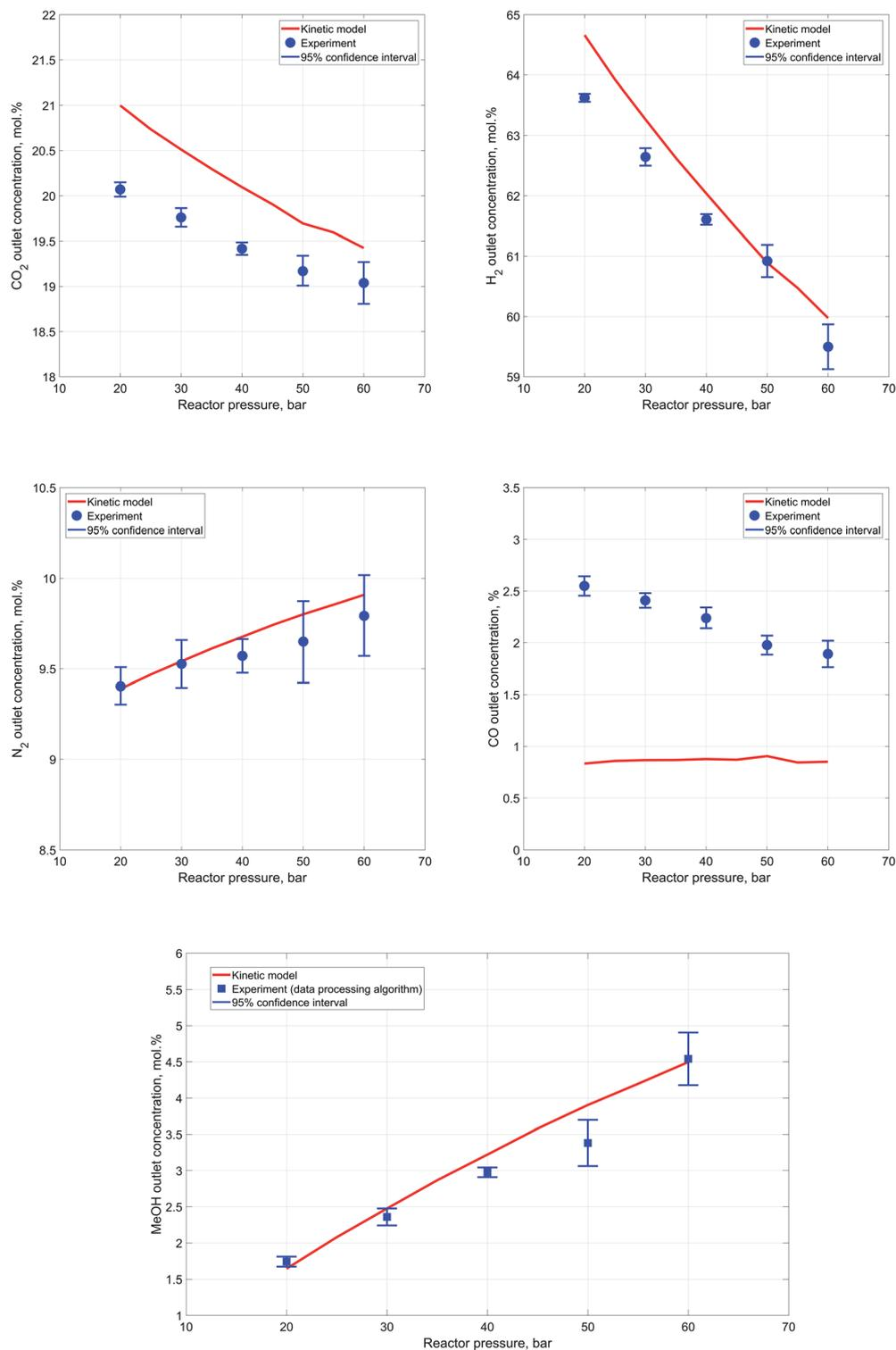
Fig. 7 (a). Dependence of the outlet  $\text{CO}_2$  concentration from the reactor pressure. (b) Dependence of the outlet  $\text{H}_2$  concentration from the reactor pressure. (c) Dependence of the outlet  $\text{N}_2$  concentration from the reactor pressure. (d) Dependence of the outlet CO concentration from the reactor pressure. (e) Dependence of the outlet MeOH concentration from the reactor pressure.
