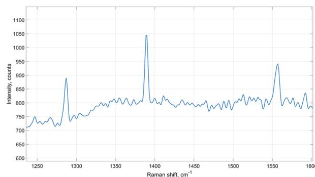
Fig. 6 Raman signals of carbon dioxide and oxygen (1555 cm<sup>-1</sup>) detected during catalyst activation (reactor temperature 180 °C, ambient pressure).
