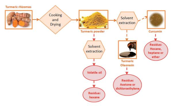
Fig. 1 Process flow diagram for the conventional turmeric processing chain.<sup>9</sup>
