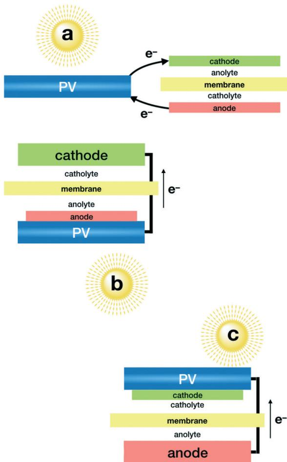
**Fig. 1** Plausible schemes for the conversion of sunlight, CO<sub>2</sub> and H<sub>2</sub>O to fuels based on a PV plus unbiased electrolyser architecture: a) simple wired PV plus an electrolyser; b) and c) integration of the PV module as a support for a cathode or an anode, to drive both reactions through the wired counter electrode.
