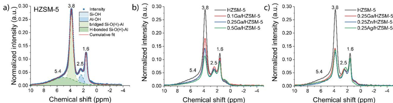
**Fig. 1**  $^1\text{H}$  MAS NMR spectra of a) parent HZSM-5; b)  $x\text{Ga}/\text{HZSM-5}$  and c)  $0.25\text{Ga}/\text{HZSM-5}$ ,  $0.25\text{Zn}/\text{HZSM-5}$  and  $0.25\text{Ag}/\text{HZSM-5}$  as compared to the parent HZSM-5 zeolite. The peaks with a chemical shift of 3.8 ppm and 5.4 ppm correspond to isolated and H-bonded bridged Si-O(H)-Al respectively. The signals at 2.5 ppm and 1.6 ppm are assigned to extra-framework Al-OH and Si-OH groups, respectively.
