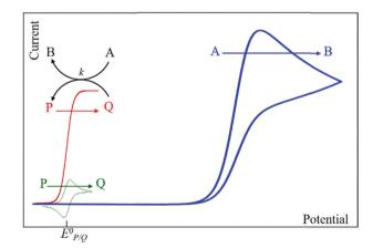
Fig. 2 Canonical cyclic voltammograms for the molecular catalysis of a one-electron catalytic electrochemical reaction (blue: direct reduction of A; green: reversible one-electron reduction of P in the absence of A; red: catalytic reduction of A triggered by the reduced form of the catalyst Q). Adapted from ref. 15 with permission from Wiley. Copyright 2006.
