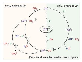
Fig. 8 Proposed mechanism of CO<sub>2</sub> reduction with Co27. During CPE at the Co<sup>II/I</sup> wave, trace amounts of CO were released. A formal oxidation state is given for the different Co species. Reprinted with permission from ref. 41. Copyright (2020) American Chemical Society.
