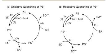
**Scheme 4** Photosensitizer (PS) emission quenching pathways. EA: electron acceptor (catalyst or electron mediator), SD: sacrificial electron donor.
