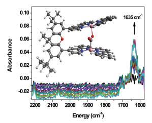
Fig. 14 Infrared spectro-electrochemistry data on a 1 mM solution of  $Co_23$  in CH<sub>3</sub>CN (0.1 M <sup>n</sup>Bu<sub>4</sub>NPF<sub>6</sub>, 0.5 M TEA) under CO<sub>2</sub> at potentials between  $-0.35\ V$  and  $-0.85\ V$  vs. Ag pseudo-reference. Inset: Calculated structure of the CO<sub>2</sub>-reduced complex adduct identified at 1635 cm<sup>-1</sup>. Adapted with permission from ref. 40. Copyright 2019, Springer Nature.
