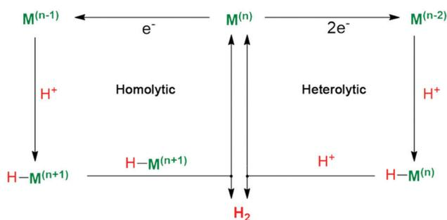
Fig. 9 Proposed mechanistic pathways for H<sub>2</sub> evolution by a metallic catalytic center.
