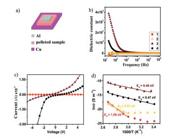
Fig. 6 (a) Fabrication of an electronic device for dielectric and electrical measurements. (b) Frequency-dependent dielectric constants of 1–4 recorded at room temperature. (c) Current-voltage curves recorded at room temperature. (d) Temperature-dependent electrical conductivity; straight lines represent Arrhenius fitting to the experimental data.
