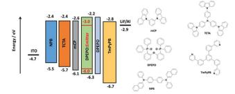
Fig. 8 Chemical structures and energy levels of materials used for the device fabrication
