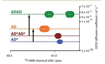
Fig. 7 Overlay of the <sup>19</sup>F NMR DOSY (400 MHz, TCE-d<sub>2</sub>, 298 K, *ca.* 5 mM) spectra of AD, AD\*, ADAD, and AD\*AD\*. Arrows highlight the decrease in the diffusion coefficient due to intermolecular hydrogen bonding interactions involving the phenols in AD and ADAD. In AD\*AD\*, the two <sup>19</sup>F signals are not resolved.
