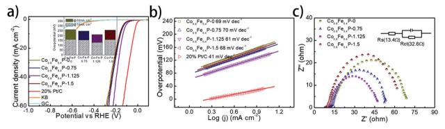
Fig. 4 (a) Polarization curves of  $Co_{0.6}Fe_{0.4}P$  and control samples for the HER in 1.0 M KOH (inset: the column diagram of HER activities for all  $Co_{0.6}Fe_{0.4}P$  catalysts); (b) the corresponding Tafel plots of all the  $Co_{0.6}Fe_{0.4}P$  catalysts and 20% Pt/C; (c) Nyquist plots of all  $Co_{0.6}Fe_{0.4}P$  catalysts at -0.15 V over the frequency range from 100 000 to 0.01 Hz.
