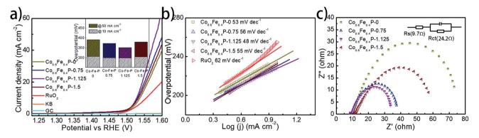
Fig. 5 (a) Polarization curves of  $Co_{0.6}Fe_{0.4}P$  and control samples for the OER in 1.0 M KOH (inset: the column diagram of OER activities for all Co<sub>0.6</sub>Fe<sub>0.4</sub>P catalysts); (b) the corresponding Tafel plots of all the Co<sub>0.6</sub>Fe<sub>0.4</sub>P catalysts and RuO<sub>2</sub>; (c) Nyquist plots of all Co<sub>0.6</sub>Fe<sub>0.4</sub>P catalysts at -1.53 V over the frequency range from 100 000 to 0.01 Hz.
