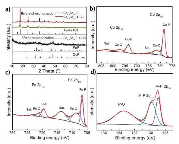
Fig. 2 (a) Powder XRD patterns of the  $Co_{0.6}Fe_{0.4}PBA$  before and after etching, and the  $Co_{0.6}Fe_{0.4}P-1.125$  after phosphorization; high-resolution XPS (b) Co 2p, (c) Fe 2p, (d) P 2p spectra of the  $Co_{0.6}Fe_{0.4}P-1.125$ .
