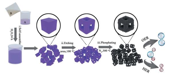
Fig. 1 Schematic illustration of the preparation of the nanoframes composed of  $Co_{0.6}Fe_{0.4}P$  NPs coated with the carbon matrix. (i) Self-assembly of Co-Fe PBA; (ii) etching of the Co-Fe PBA to produce nanocages; (iii) phosphidation of the Co-Fe PBA nanocages to obtain subsequent Co<sub>0.6</sub>Fe<sub>0.4</sub>P NPs coated with the carbon matrix.
