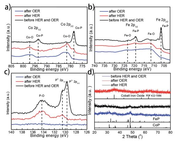
Fig. 7 High-resolution (a) Co 2p, (b) Fe 2p, and (c) P 2p XPS spectra of the as-prepared, post-HER and post-OER Co<sub>0.6</sub>Fe<sub>0.4</sub>P-1.125 catalysts; (d) XRD patterns of the as-prepared, post-HER and post-OER Co<sub>0.6</sub>Fe<sub>0.4</sub>P-1.125 catalysts
