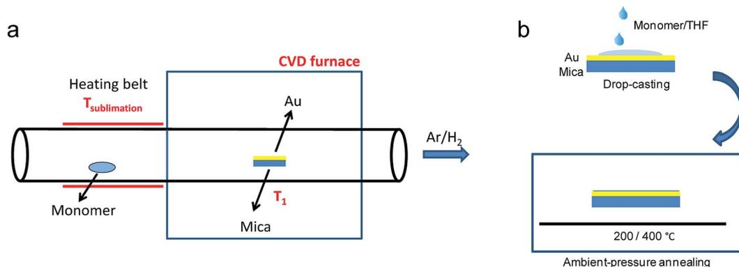
Fig. 4 Schematic illustration comparing GNR synthesis through (a) CVD and (b) solution processing, which avoids the use of heat and vacuum for the monomer deposition. (a) Reproduced with permission.<sup>66</sup> Copyright (2016) American Chemical Society; (b) Reproduced with permission.<sup>120</sup> Copyright (2017) The Chemical Society of Japan.
