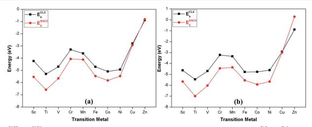
Fig. 2  $E_b^{SAC3}$  and  $E_b^{SAC4}$  are the binding energies of embedded three and four metal atoms with the B<sub>β12</sub> monolayer.  $E_b^{CL3}$  and  $E_b^{CL4}$  are the binding energies of metal clusters (comprised of three and four metal atoms) with the B<sub>β12</sub> monolayer.
