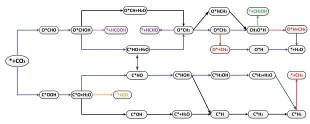
Scheme 1 Most likely reaction pathways for the electroreduction of CO<sub>2</sub> on TM-B<sub>B12</sub>.
