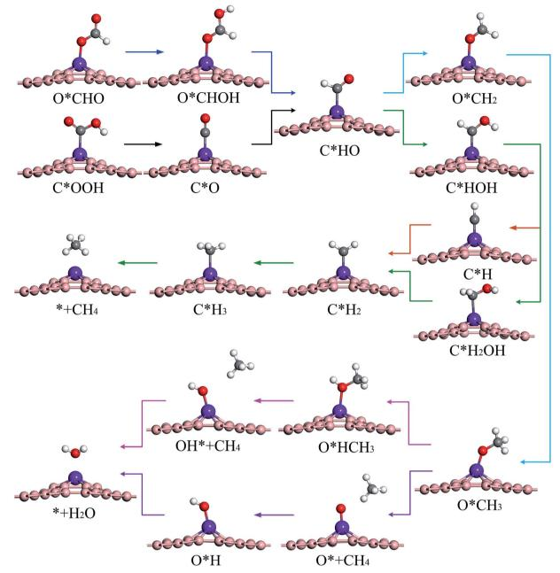
Fig. 4 Optimized geometric structures of key reaction intermediates of CRR.
