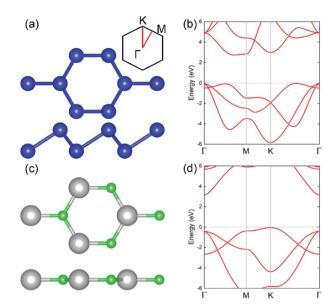
Fig. 3 Top and side views of (a) BlueP and (c) g-GaN. Band structures obtained by HSE06 of (b) BlueP and (d) g-GaN. The blue, gray, and cyan spheres represent P, Ga, and N atoms, respectively; the Fermi level is represented by the gray dashed line.
