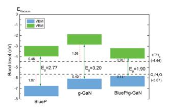
Fig. 5 Band-edge alignment, obtained by HSE06, of BlueP monolayer, g-GaN monolayer, and g-GaN/BlueP vdW heterostructure. The potentials of oxidation ( $O_2/H_2O$ ) and reduction ( $H^+/H_2$ ) at pH = 0 for water splitting are also shown.
