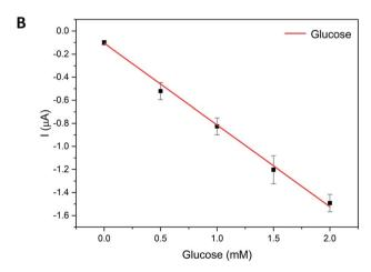
Fig. 5 Amperometric detection of glucose in the flow injection analysis system with 3D-PMED. (A) Amperometric current response at  $-0.1 \,\mathrm{V}$  (vs. Ag/AgCl reference electrode) with alternant injecting of glucose (successive addition of 0.5 mM, 1.0 mM, 1.5 mM, 2.0 mM glucose) and PBS. (B) The calibration plot with the error bar ranging from 0 mM to 2.0 mM.
