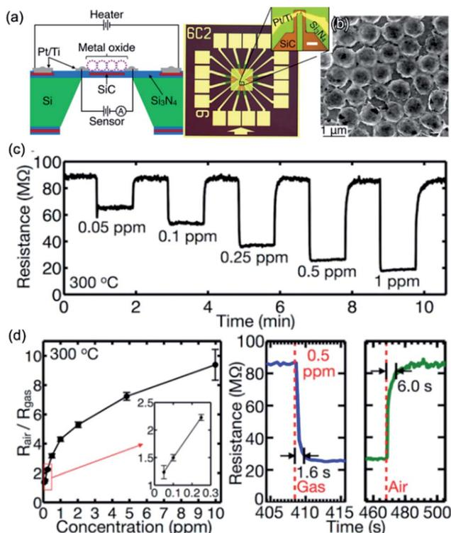
Fig. 7 (a) Schematic diagram and (b) morphology of the as-fabricated sensor with the integration of microheater platform and macroporous  $\text{SnO}_2$  hollow spherical array. (c) Real-time sensor resistance transient to HCHO at 300 °C. (d) Sensor response versus HCHO concentration, and real-time sensor response and recovery behaviors to 0.5 ppm HCHO. Reproduced with permission.<sup>84</sup> Copyright 2017, American Chemical Society.
