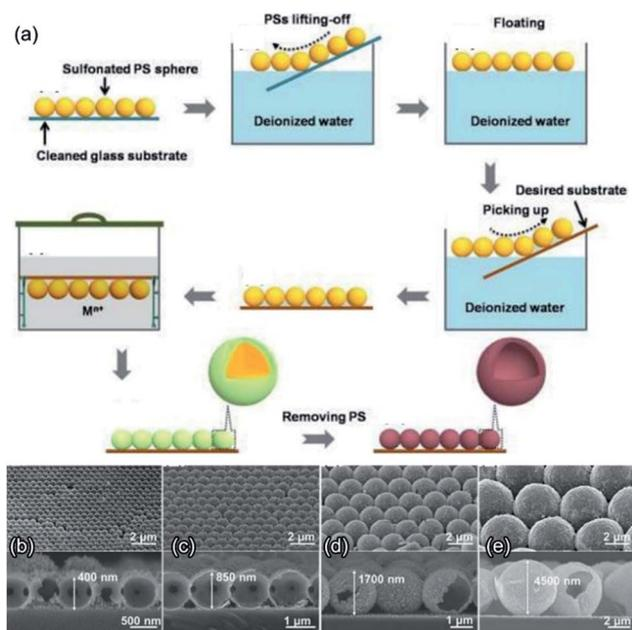
Fig. 2 (a) Schematic illustration of the formation process of ordered metal oxide macroporous hollow spherical arrays. (b–e) Fabricated  $\text{Fe}_2\text{O}_3$  hollow spherical arrays with different aperture sizes by using 500, 1000, 2000, and 5000 nm PS spherical templates. Reproduced with permission.<sup>48</sup> Copyright 2017, Elsevier Ltd.
