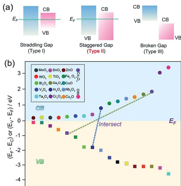
Fig. 9 (a) Three types of semiconductor heterojunctions organized by band alignment. (b) CB and VB band positions referred to the Fermi level ( $E_C - E_F$  or  $E_V - E_F$ ). In the upper portion, the CB position is arranged according to the distance to  $E_F$  for these oxides; in the bottom part, the VB position is also arranged according to the distance to  $E_F$ .
