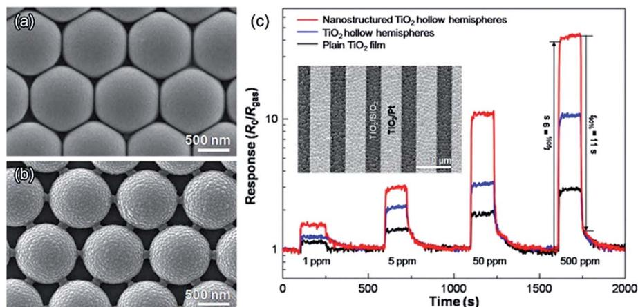
Fig. 6 Top-view SEM images of (a)  $\text{TiO}_2$  hollow hemispheres and (b) nanostructured  $\text{TiO}_2$  hollow hemispheres (pointy contact between hemispheres); (c) sensing transients of plain  $\text{TiO}_2$  film, hollow hemispheres, and nanostructured hollow hemispheres to 1–500 ppm CO at 250 °C. Reprinted with permission.<sup>82</sup> Copyright 2010, Elsevier Ltd.
