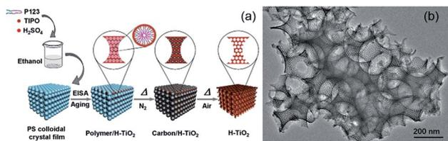
Fig. 4 (a) Schematic illustration of the formation and (b) microstructure of a hierarchically 3D ordered mesoporous-macroporous  $\text{TiO}_2$  structure. Reproduced with permission.<sup>74</sup> Copyright 2014, Wiley-VCH.
