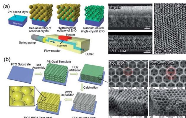
Fig. 3 (a) Flow-reactor-assisted hydrothermal fabrication process and morphologies of 3DOM  $\text{ZnO}$ . Reproduced with permission.<sup>52</sup> Copyright 2017, American Chemical Society. (b) Fabrication process and morphologies of core-shell 3DOM  $\text{TiO}_2$  and  $\text{TiO}_2$ - $\text{WO}_3$ . Modified with permission.<sup>53</sup> Copyright 2018, Royal Society of Chemistry.
