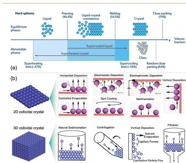
Fig. 1 (a) Phase diagrams of monodisperse colloids at different volume fractions. Modified with permission.<sup>36</sup> Copyright 2016, Macmillan Publishers Limited. (b) 2D and 3D crystallization methods for close-packed CCs.
