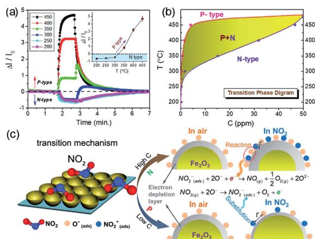
Fig. 8 (a)  $\text{NO}_2$  response of 2DOM  $\text{Fe}_2\text{O}_3$  at different temperatures ( $T$ ) and concentrations ( $C$ ). (b)  $T$ - $C$  transition phase diagram. (c) Schematic illustration of different  $\text{NO}_2$  sensing types at high and low  $C$  values, respectively. Reproduced with permission.<sup>98</sup> Copyright 2015, Royal Society of Chemistry.
