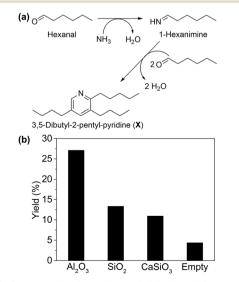
Fig. 1 (a) Scheme for formation of 3,5-dibutyl-2-pentyl-pyridine (compound X) and (b) yield of compound X with different supports. Reaction conditions: 1 μL min<sup>-1</sup> hexanal, 200 mg catalyst, 190 °C, 8 mL  $min^{-1} NH_3$ , 20 mL  $min^{-1} N_2$ . GHSV = 1.12 × 10<sup>4</sup> h<sup>-1</sup>.
