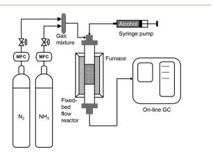
Scheme 1 Experimental set-up for the conversion of alcohols to
