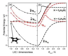
Fig. 4 Singlet (in black) and triplet (in red) PECs for  $C_6H_6$ . Panel (a) is for a sequence of geometries along a LIIC connecting the optimised ground state geometry to that of the prefulvenic MECI linking the  $^1\pi\pi^*$  and  $S_0$  PESs, the structure of which is included as an inset. The PECs shown in panel (b) are from a rigid body scan wherein  $R_{C-H}$  is extended at planar geometries with the rest of the nuclear framework fixed at its ground state equilibrium geometry.
