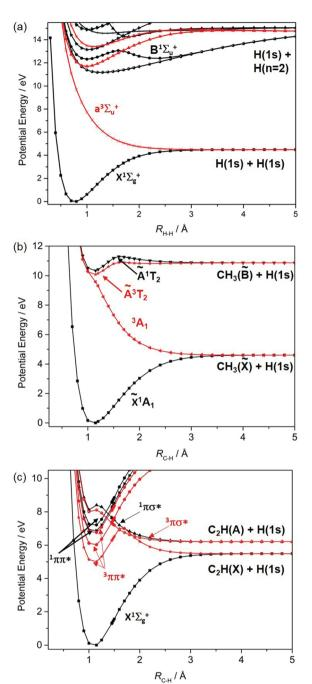
Fig. 1 Singlet (in black) and triplet (in red) PECs for (a) H2 and, as a function of  $R_{C-H}$ , for (b) CH<sub>4</sub> and (c) HCCH. The latter two sets of curves are rigid body scans, calculated by progressively extending one C-H bond while holding the rest of the nuclear framework fixed at its ground state equilibrium geometry, with the constraint that the overall symmetry remains as  $C_{3v}$  and  $C_{\infty v}$ , respectively
