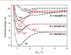
**Fig. 3** Rigid body singlet (in black) and triplet (in red) PECs for HCHO plotted as a function of  $R_{\rm C-H}$  for planar geometries, with the rest of the nuclear framework maintained at its ground state equilibrium geometry.
