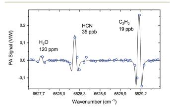
Fig. 3 Measured and simulated 2<sup>nd</sup> harmonic spectra with the optical build-up cavity for the PA signal enhancement.
