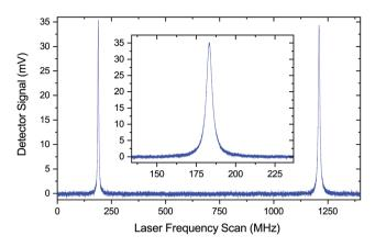
Fig. 2 Cavity transmission spectrum over two longitudinal cavity modes as a function laser frequency scan. The spectrum was measured with a narrow linewidth laser and a fast photodetector. Inset: Zoom over a cavity mode.
